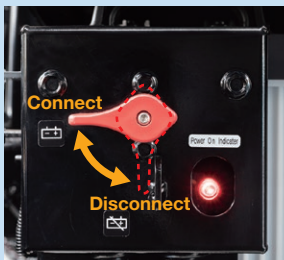
Battery Disconnect Switch
