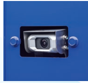
Right front view camera
