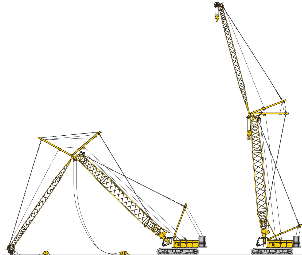
Erecting of main boom and luffing jib
