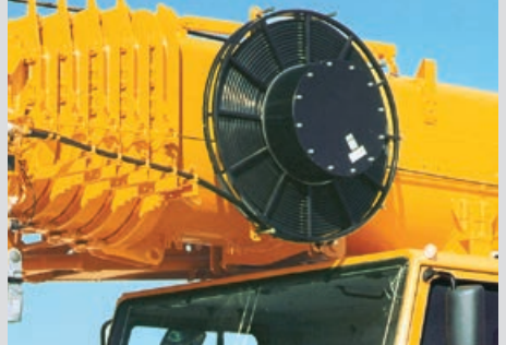
Hose drum for hydraulic cylinder
