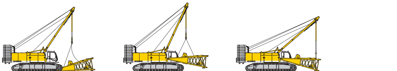
Unloading and assembly of boom foot
