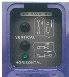
Jib assist cylinder control switch
