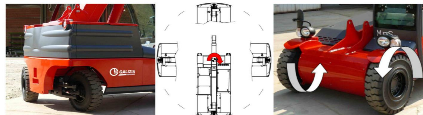
**front wheel drive with 2 motors and counter rotation - total steering**
