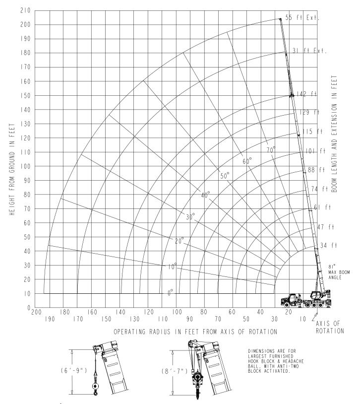
\*THIS DRAWING SHOWS THE PHYSICAL REACH OF THE MACHINE. ALWAYS REFER TO LOAD CHART TO SEE WHICH PORTIONS OF THIS DIAGRAM ARE VALID FOR THE SPECIFIC MACHINE CONFIGURATION.
