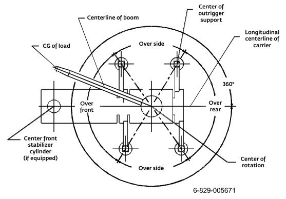
Bold lines determine the limiting positon of any load for operation within working areas indicated.
