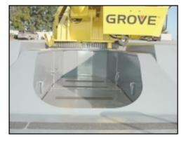
Large open stowage compartment for tools and rigging accessories
