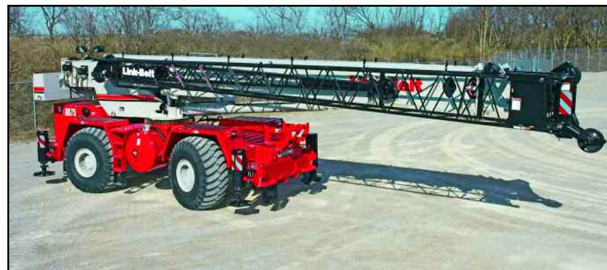
A-max extends only the inner-mid section of the boom for substantially increased capacities for in-close, maximum capacity lifts.
