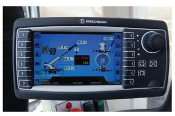
The convenient LMAP menu navigation with an intuitive user interface displays load on hook, rated capacity percentage, boom length and angle, load radius, and operator-defined protection with audible alarms. While the intuitive display and user interface are unique to Altec, the system's hardware consists of common "off-the-shelf" components that were critically selected for their performance and serviceability.
