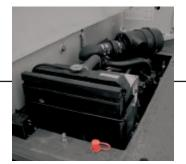
**Cummins engine** The Cummins QSB 3,3 L, Tier III, diesel comes **standard** in both models.
