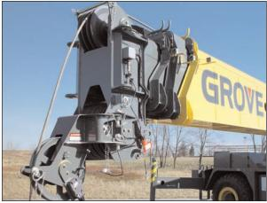
The RT530E-2 incorporates a rectangular boom shape made from 100k.s.i. steel which eliminates weight and maximizes structural capacities.
