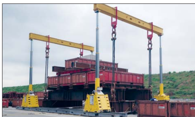
◀ SL400 Gantry during load testing.
