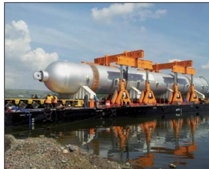
Offloading a 1,300-Ton Hydrocracker
