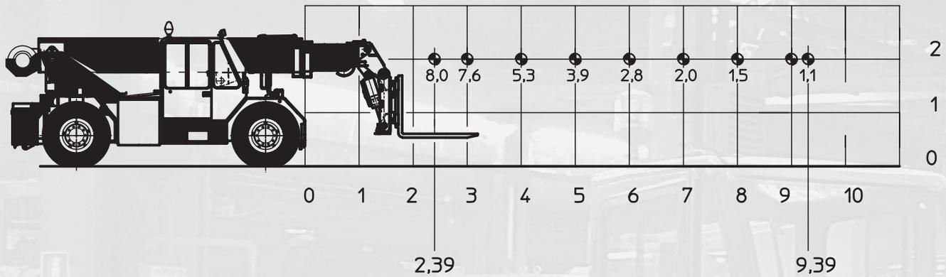
Lifting capacity chart with fly-jib (tonnes)
