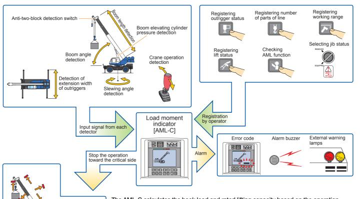
The AML-C calculates the hook load and rated lifting capacity based on the operation state registered by the operator and input signal from each detector, and displays them as a moment load ratio. When the moment load ratio reaches or exceeds 100%, the AML-C stops the crane operations toward the critical sides and warns with error codes and a buzzer. (The AML-C is a safety device that aids the operator in preventing accidents, such as machine overturn, and damage resulting from overload.)
