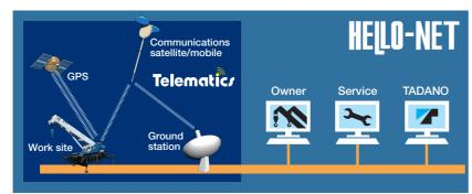
Telematics (machine data logging and monitoring system) with HELLO-NET via internet (\*availability depends on the situation). DETAILS: The availability of data communication systems, such as satellite or mobile communications which serve to widen the service area differs according to individual countries. Besides, there are some countries where the system itself is not in use yet.
