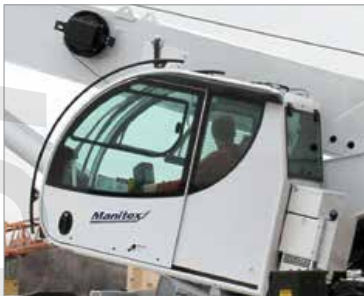
Operator cab tilts from 0° to 20° for a comfortable, clear view of the load.
